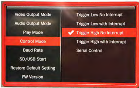
Proper setting for a PIR sensor shown Step mats use "Trigger Low No Interrupt"
